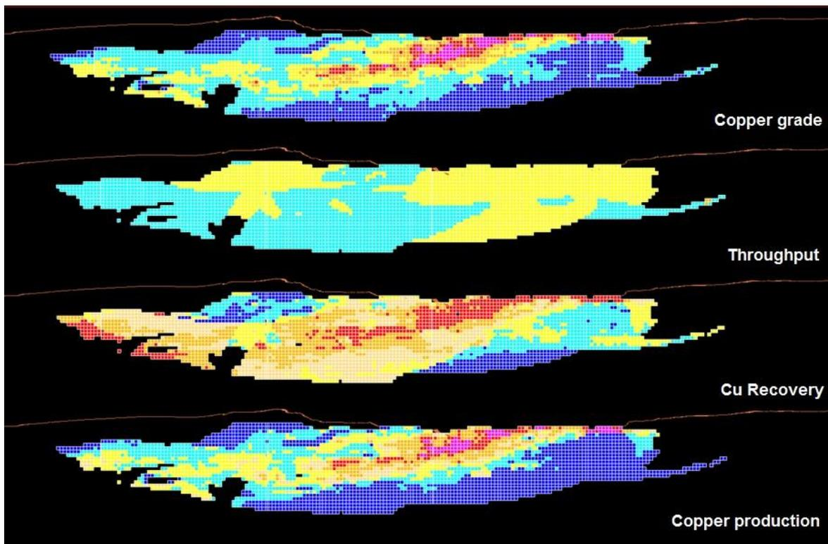
**Figure 5** From top to bottom: Sections of MMIC pit showing copper grades, throughput, copper recovery, and total copper production at a fixed P80 (250  $\mu\text{m}$ )
